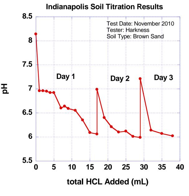
Response of well buffered soil to 0.725 N HCl addition
