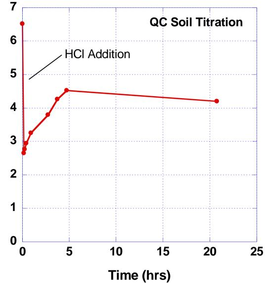
Response of poorly buffered soil to addition of 1 mL of 0.725 N HCl
